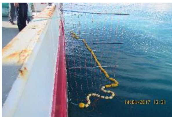
Figure 14 FV Tronio bird exclusion device (BED) around the hauling bay.
