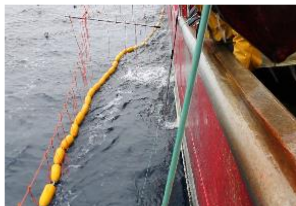
Figure 15 FV Tronio bird exclusion device (BED) around the hauling bay.
