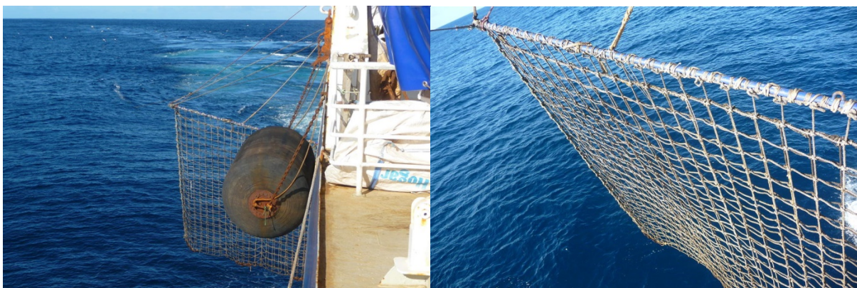
Figure 2: The side fence of the bird repeller used on the RTMKSm "Admiral Shabalin"
