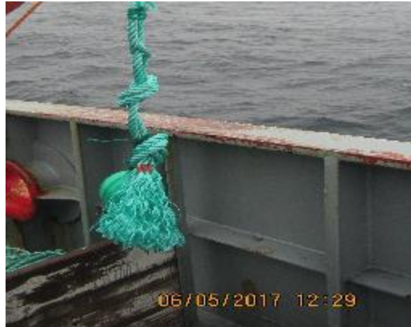
Figure 20: Towed device option 2, providing additional drag
