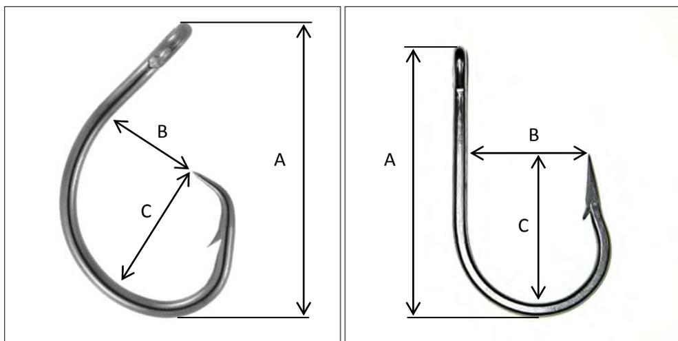
**Figure 3** planes of measurement for both Circle (Left) and J-hooks (Right). A- total Length, B- Gape, C- Bite / Throat
